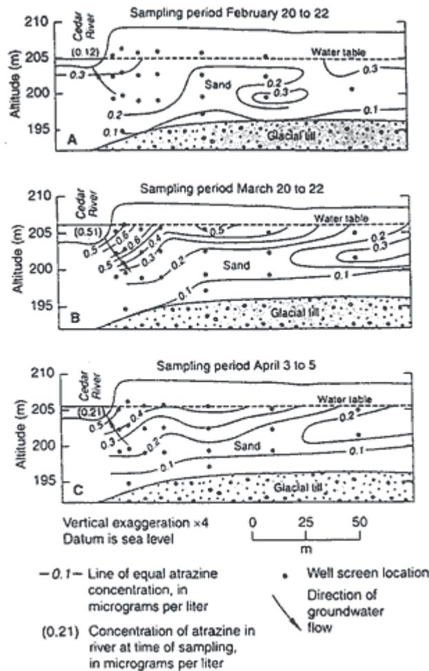
**Figure 17 A-C** Hydrogeologic sections for part of the Cedar River, Iowa, for three time periods in 1990. **A** Movement of groundwater into the river prior to a period of high river stage. **B** Movement of river water into the contiguous aquifer during high river stage. **C** Return of some of the water from the aquifer during declining river stage. (Modified from Squillace et al. 1993)
