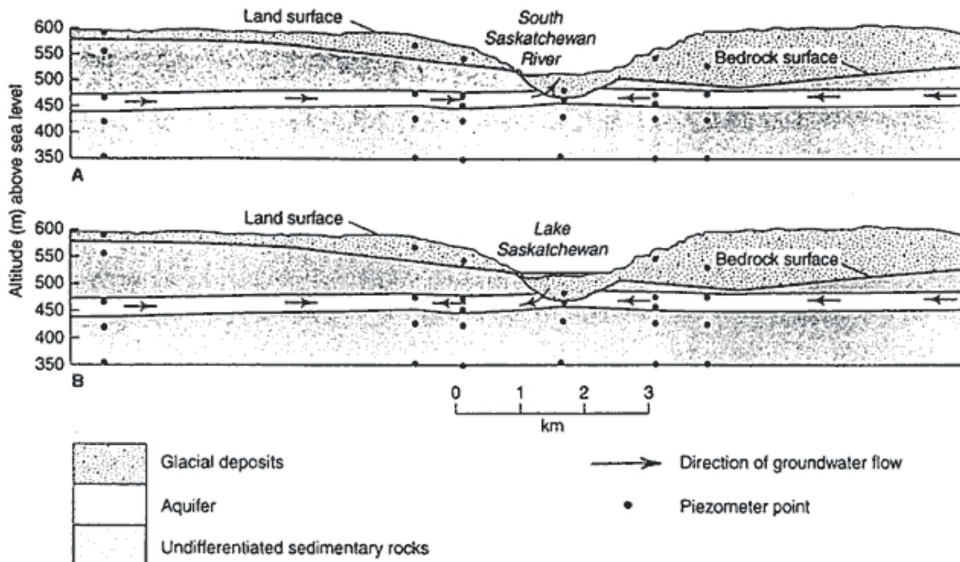
**Figure 7A,B** Hydrologic section across the Saskatchewan River, Canada. **A** Groundwater flow in a bedrock aquifer before construction of a reservoir on the South Saskatchewan River. **B**, Reversal of flow in part of the aquifer following filling of the reservoir. Only the principal aquifer is shown. (Modified from van Everdingen 1967)
