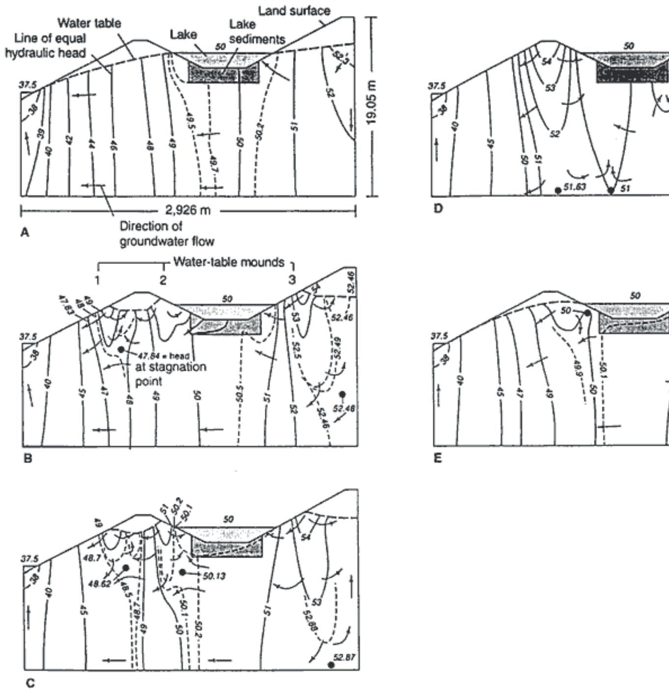
**Figure 4 A-E** Distribution of hydraulic head and direction of groundwater flow for variably saturated porous media near surface water. Beginning with a steady-state water table **A**, results are of conditions following 5 days **B**, 10 days **C**, and 15 days **D** of infiltration. **E** Conditions after 7 months of redistribution. (Modified from Winter 1983)
