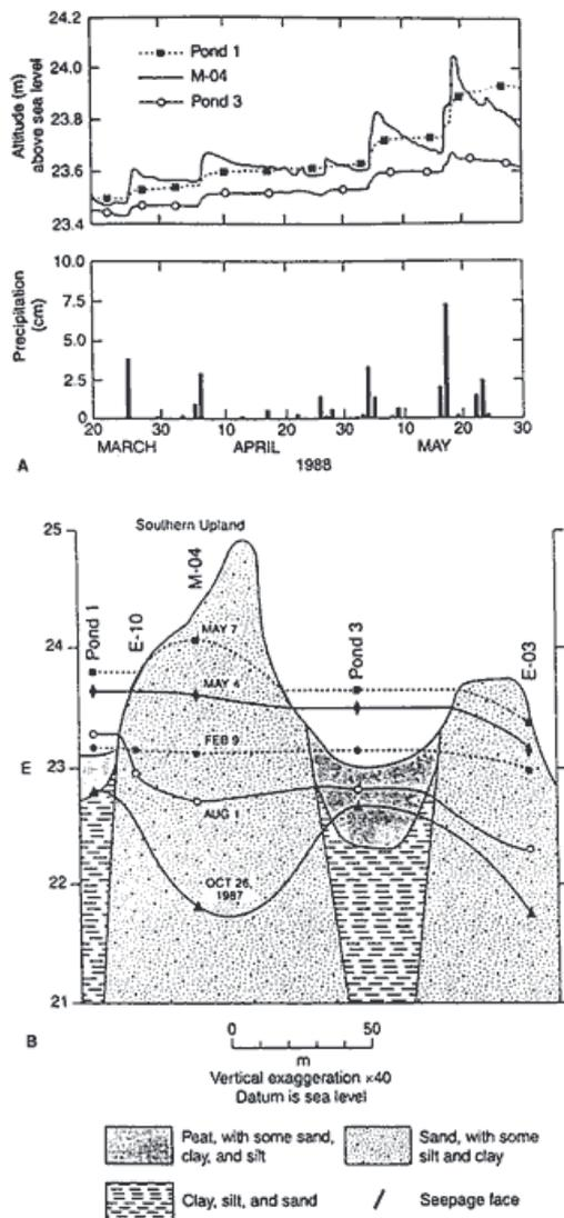
**Figure 15 A,B** Hydrologic conditions near seasonal ponds on the Atlantic Coastal Plain, Delaware. **A** Hydrographs showing responses of two ponds and one well to precipitation during spring of 1988. **B** Profiles of the water table for October 21, 1987, and for several dates in 1988. (Modified from Phillips and Shedlock 1993)
