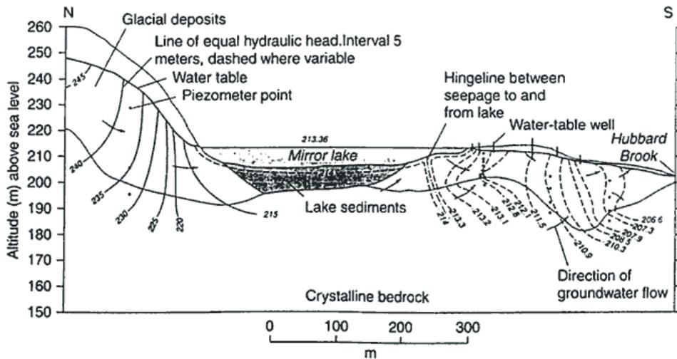
**Figure 9** Hydrologic section showing groundwater flow in the Mirror Lake area, New Hampshire
