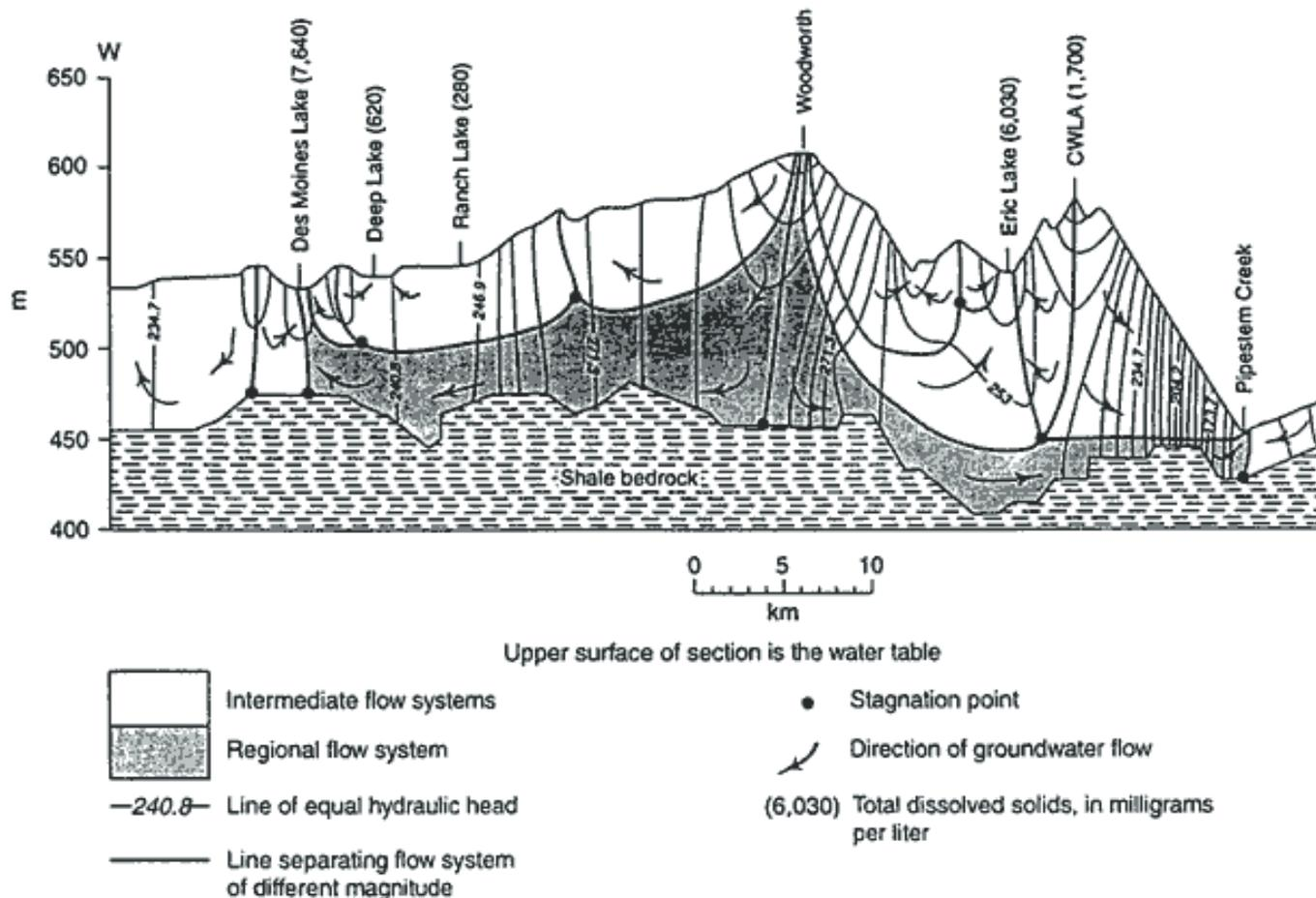
**Figure 6** Numerical model of groundwater flow through part of the Missouri Coteau in Kidder and Stutsman Counties, North Dakota, showing high values of total dissolved solids in lakes receiving groundwater discharge from regional (Des Moines Lake) and deep intermediate (Eric Lake) flow systems (Modified from Winter and Carr (1980))
