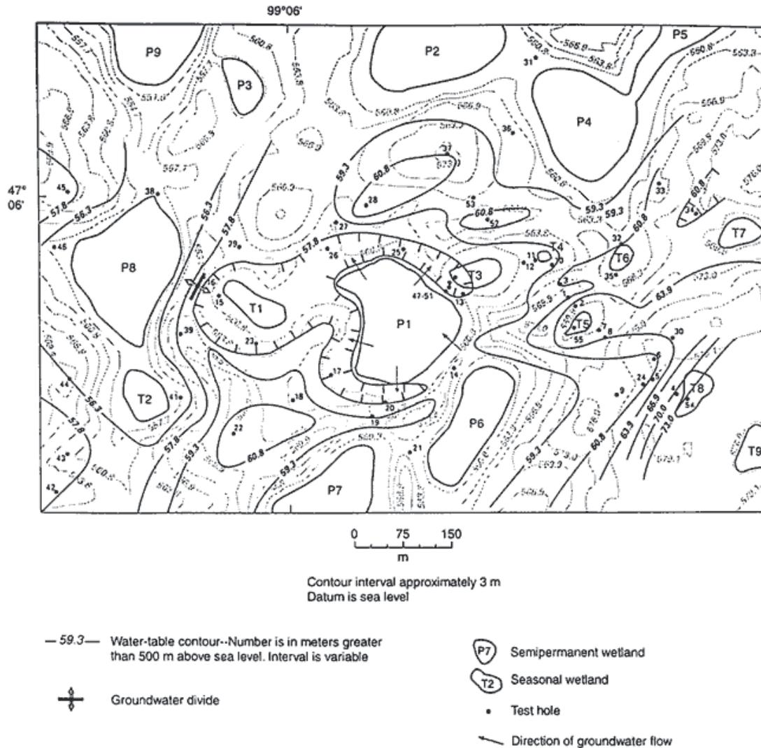
**Figure 12** Configuration of the water table in the Cottonwood Lake area, North Dakota, for August 31, 1989, showing the water-table depression around much of the perimeter of wetland P1 caused by transpiration directly from groundwater. (After Winter and Rosenberry 1995)
